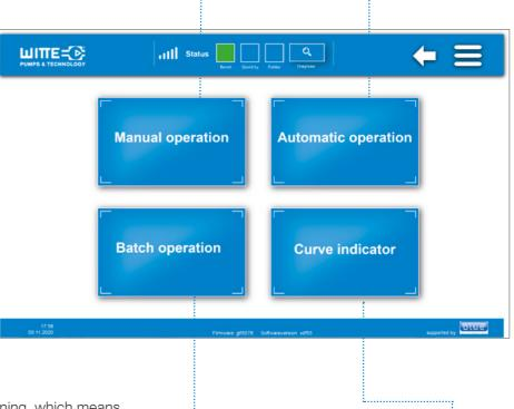
The batch mode is self-learning, which means that the controller takes into account, for example, the overrun of the pump after shutdown and compensates accordingly.
