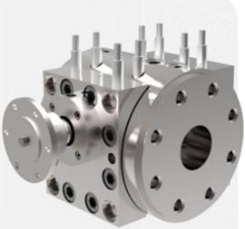
The WITTE - quick color change version lends itself particularly to master batch applications with frequent changes of color. In order to prevent the pump's drive shaft from being driven/pushed out of the housing when the suction pressure exceeds 10 bar (extruder conveying pressure), the drive shaft must be pressurewise relieved. It protrudes from both sides of the housing and is sealed, so that atmospheric pressure predominates on both sides of the drive shaft.
